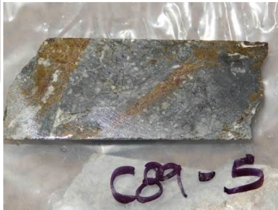
Plate 6: Example of red-brown sphalerite with pyrite and minor galena, from Hole C89-05, Duncan Lake property
