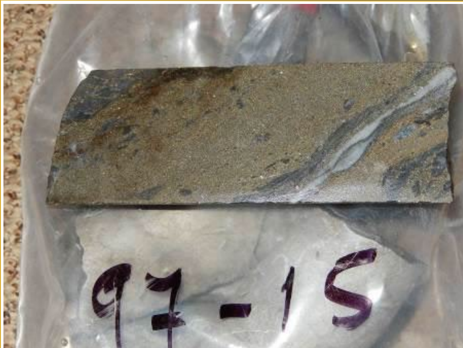
Plate 5: Example of semi-massive to massive pyrite with minor sphalerite and galena from Hole C97-15, Duncan Lake property
